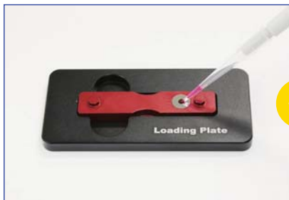
Pipette the Reference / Sample in turn.
