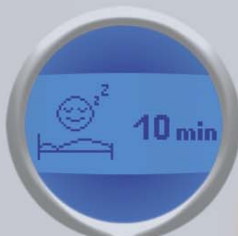
Automatic unit cut-off
