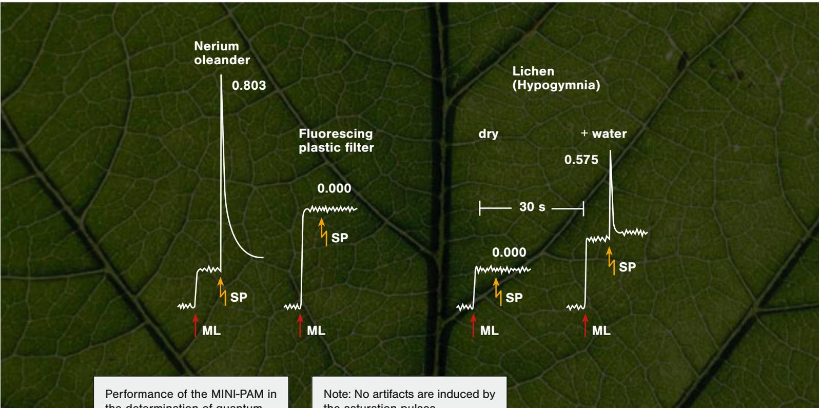
Performance of the MINI-PAM in the determination of quantum yield with different types of active and inactive samples. ML, measuring light on; SP, application of a 0.8 s saturation pulse of  $10000 \mu\text{mol m}^{-2} \text{s}^{-1}$  PAR. The numbers denote the recorded YIELD-values. Analog recording of fluorescence yield by chart-recorder.
