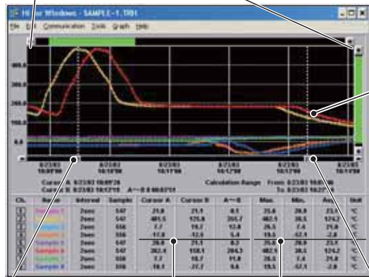
A Cursor Bar Cursor values and calculated difference Max. / Min. / Average / Unit B Cursor Bar
