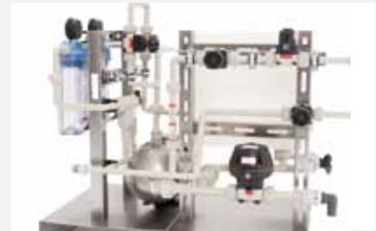
Safe, IR welded piping
