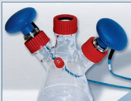
PA-housing with GL45 screwed connection on shake flask
